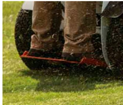
The Bobcat stand-on mowers are equipped with a robust anti-slip standing platform that can be lifted quickly and easily, so you have more control over your machine in tight spaces.
