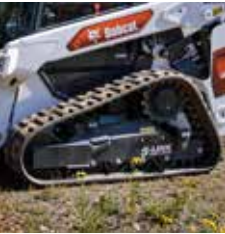
Torsion Suspension – 5 Link System
