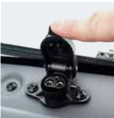
Tractor socket (12 V, 15 A)
