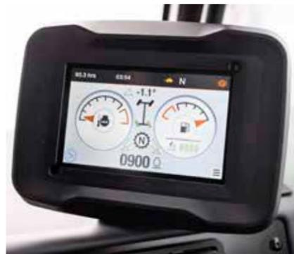
Highly readable interactive screen shows vital information in real-time. The rear view camera feed is automatically shown when reversing (optional).
